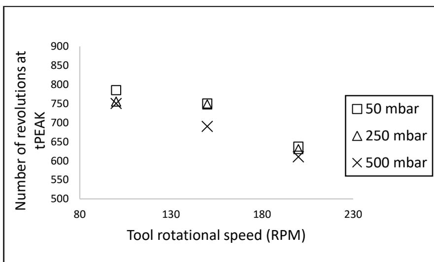
**Fig. 4: Comparison of number of spiral agitator revolutions at  $t_{PEAK}$  for different pressure levels**
