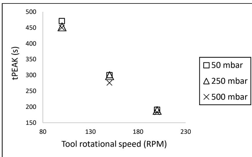
**Fig. 3: Comparison of  $t_{PEAK}$  at different pressure levels**
