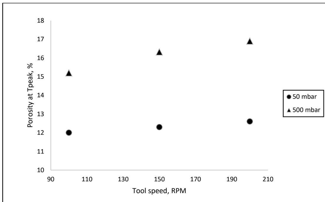
Fig. 5: Comparison of dough porosity at  $t_{PEAK}$  for different pressure levels
